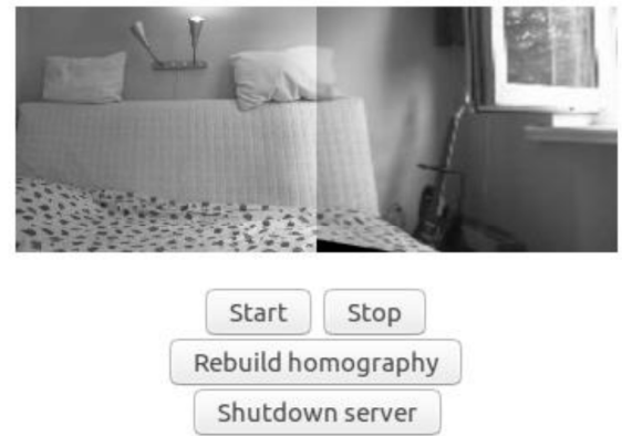
Fig. 3. Web interface with panoramic video (captured and stitched from 2 cameras)
