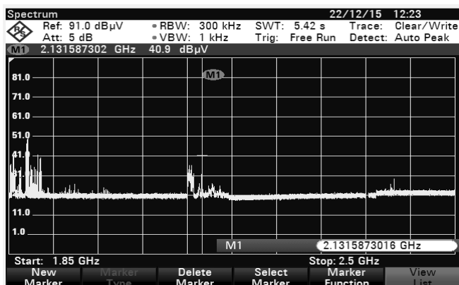
Fig. 8. Downlink 3G (2110-2170 MHz): LGS-715 Jammer is switched off (increased scale for 1.85 GHz)
