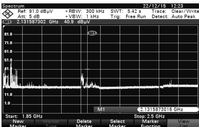
Fig. 9. Downlink 3G (2110-2170 MHz): LGS-715 Jammer is switched on (increased scale for 1.85 GHz)
