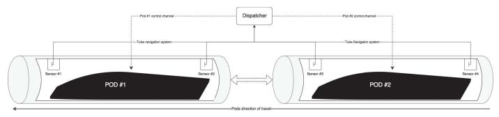
Fig. 12. Pod-Tube-Dispatcher communication system
