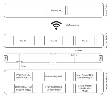
Fig. 2. System overview showing communication methods
