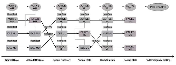
Fig. 8. MU recovery cycle. Complete transition cycle that allows for stateless recovery procedure
