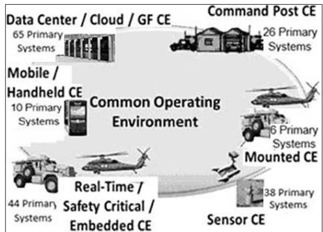
Fig. 7. COE focuses on 6 Computing Environments (CE) having 15 control points and 189 primary systems
