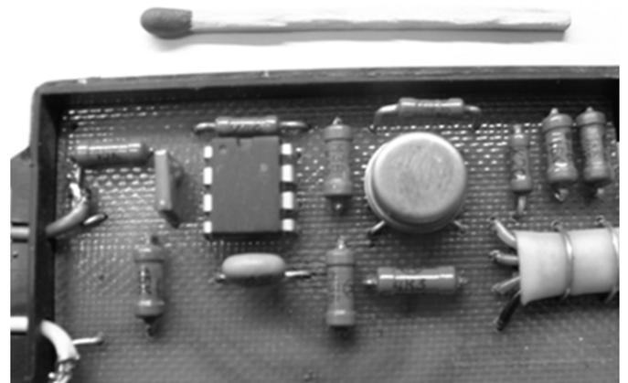
Fig. 7. Implementation of a typical scheme board of biopotential amplifier
