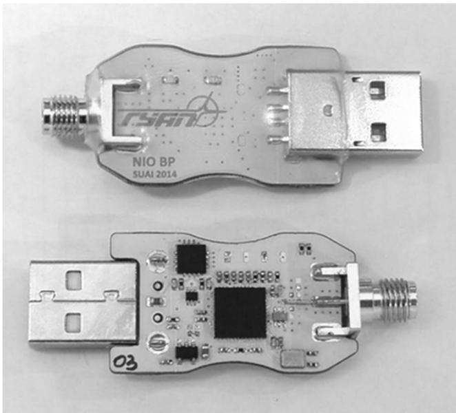
Fig. 12. Prototype of the receiving module of the implantable biotelemetric System
