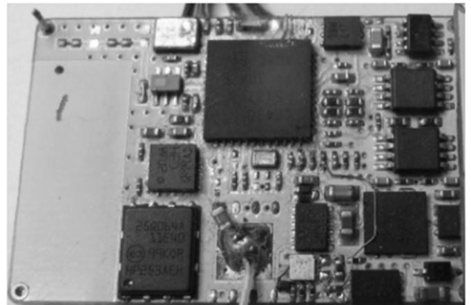
Fig. 4. The Prototype of the implantable biotelemetric system board with extended functional capabilities
