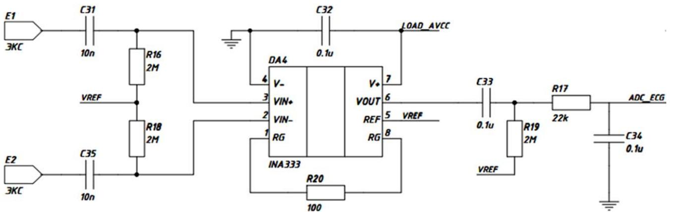
Fig. 8. Biopotential amplifier Principal Scheme of biotelemetric System's Prototype
