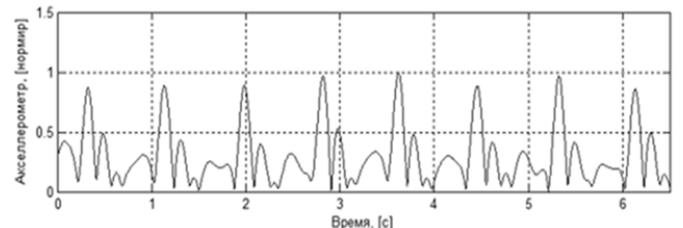
Fig. 11. The pulse wave signal recorded by accelerometer
