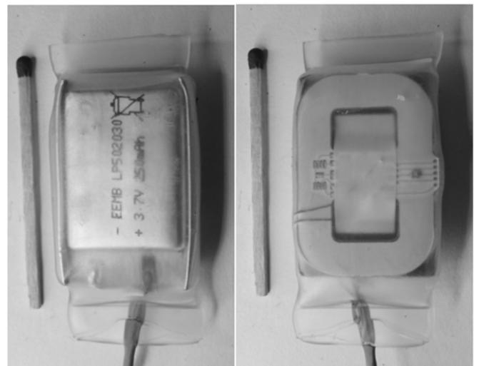
Fig. 5. The prototype of the implantable biotelemetric system in the corpus from the battery's side (left) and the receiving contour's side (right)
