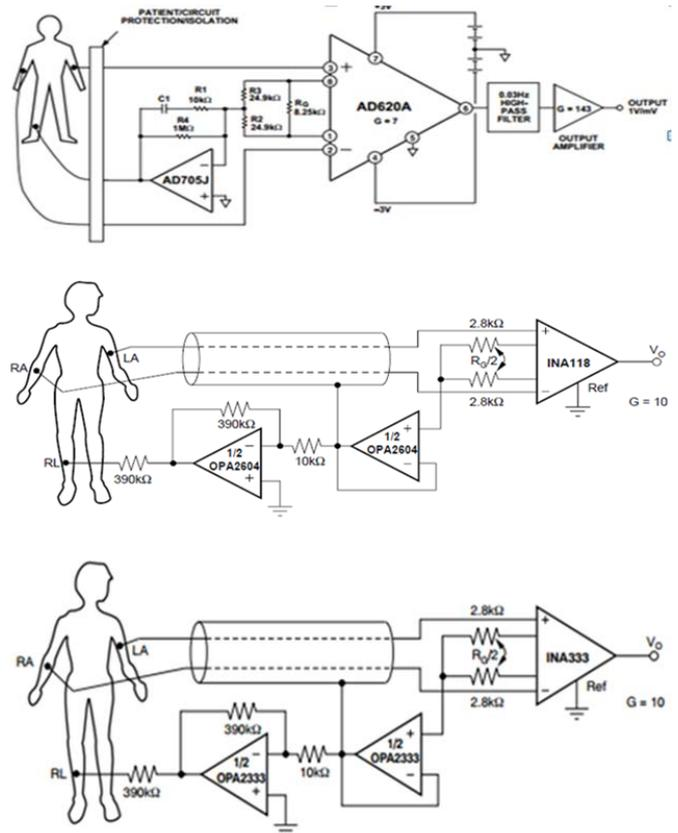
Fig. 6. Typical schemes of biopotential amplifiers (preamplifiers)
