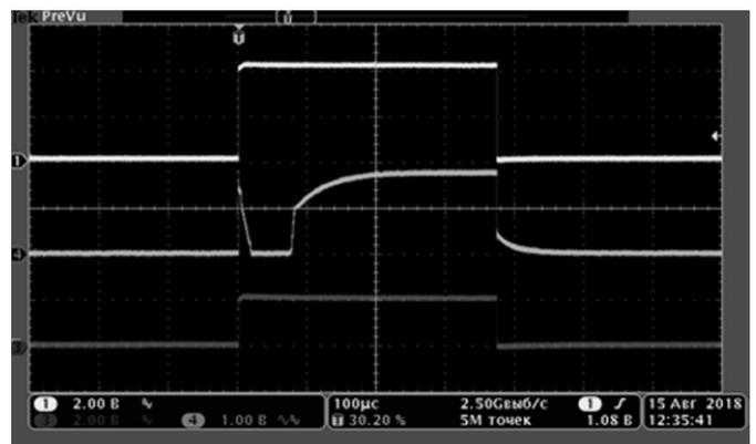
Fig. 2. Oscillograms of blood pressure sensor in pulsed power mode
