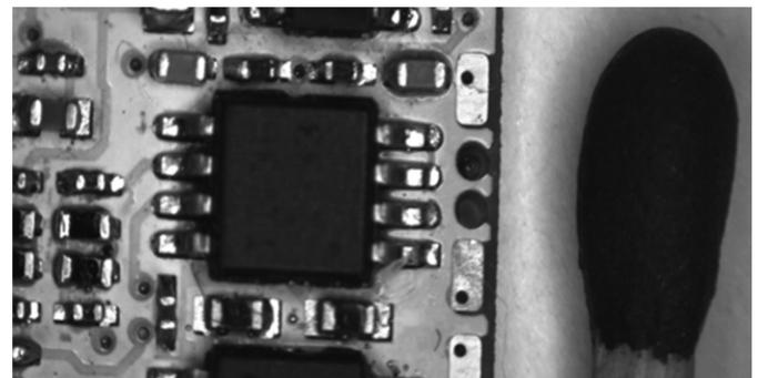
Fig. 9. Implementation of the biopotential amplifier circuit of the biotelemetric system model
