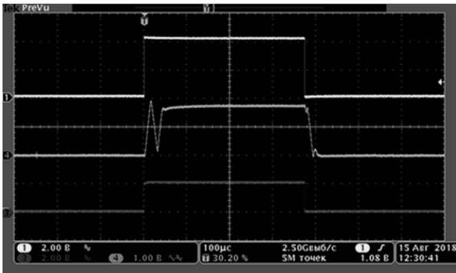
Fig. 3. Oscillogram of output signal of the amplifier of the pressure sensor signal at constant power supply of AI
