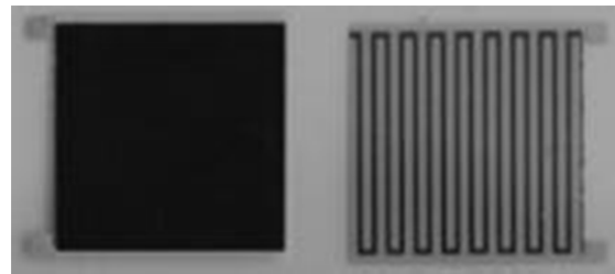
Fig. 1. Temperature sensor a) bottom side (left image) and top side (right)
