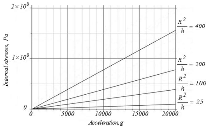
Fig.4, a. Graph of internal stresses of sensitive elements of quartz ST-cut for the proposed size relationships
