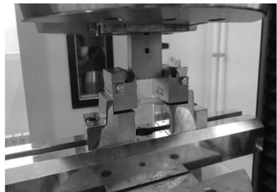
Fig.5, b. Method of fixing the plate on the equipment
