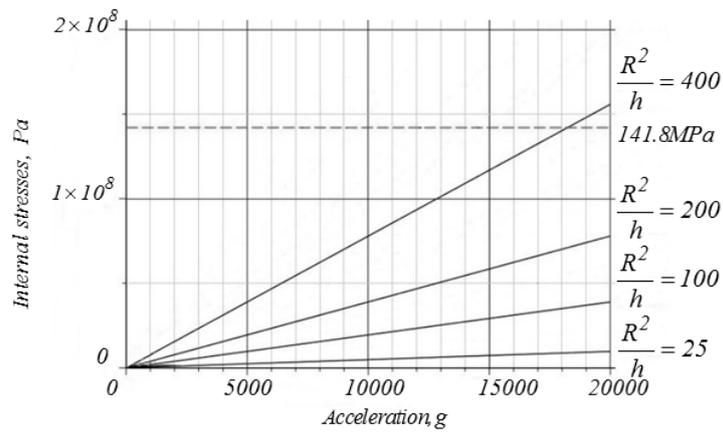
Fig. 8, a. Graph of internal stresses of sensitive elements of quartz ST-cut for the proposed size relationships
