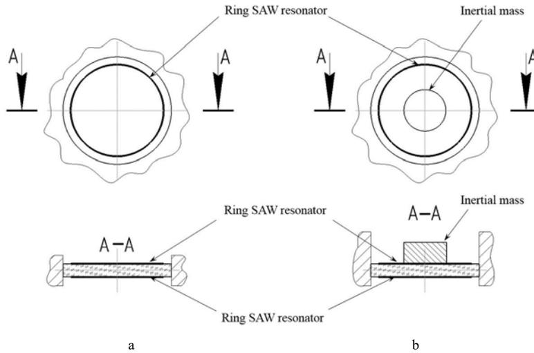
Fig.2. a. Sensitive element of a microaccelerometer on a surfactant of circular shape with a ring resonator; b. Sensitive element of a microaccelerometer on a SAW of a circular shape with a ring resonator and inertial mass in the center
