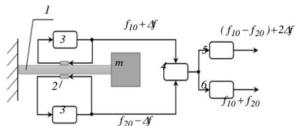
Fig.1. Structural diagram of the SAW accelerometer
