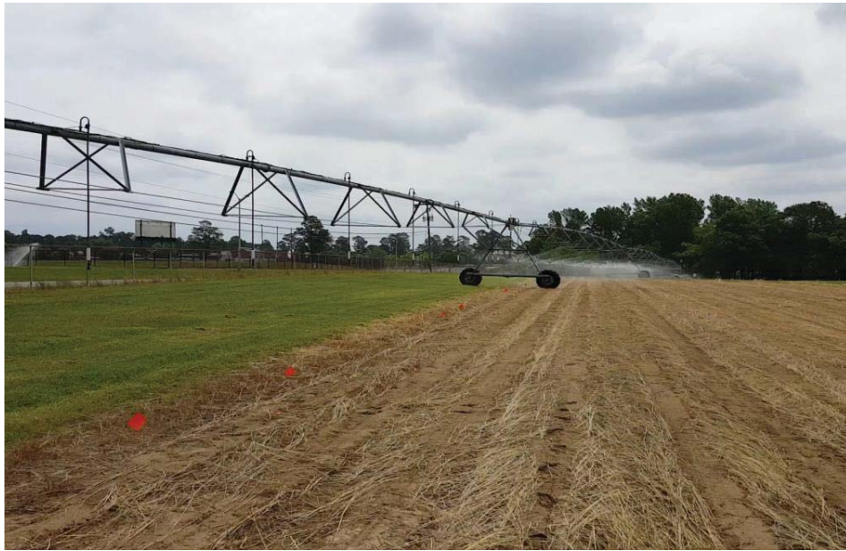
a) Variable Rate Irrigation capable center pivot (UGA, Tifton campus)
