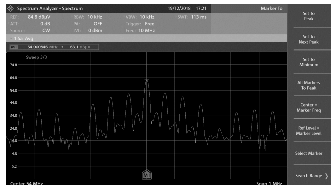
Fig. 4. Spectrogram of the compromising emanations
