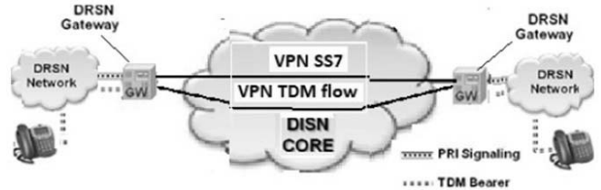
Fig. 12. A hybrid circuit-packet switching solution for DRSN
