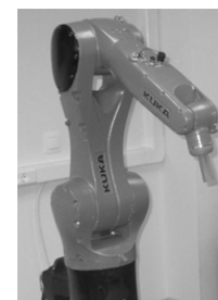
Fig. 2. KUKA palletizing robot, intended for various projects in conjunction with software and hardware controls and executive mechanisms on basis of Arduino, Raspberry Pi, and Iskra JS. Projects are aimed at working with handicapped people as well
