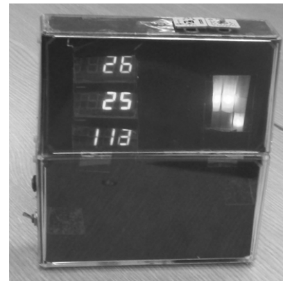
Fig. 5. System for room parameters evaluation with LED color display (weather station). The indicators on the right side of the front panel are adjusted in accordance with the sanitary and epidemiological standards for this type of premises
