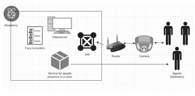
Fig. 1. Prototype architecture with main Raspberry Pi component
