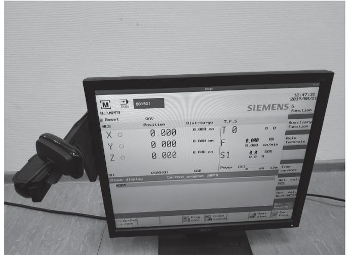
Fig. 5. Machine stand emulator: front view
