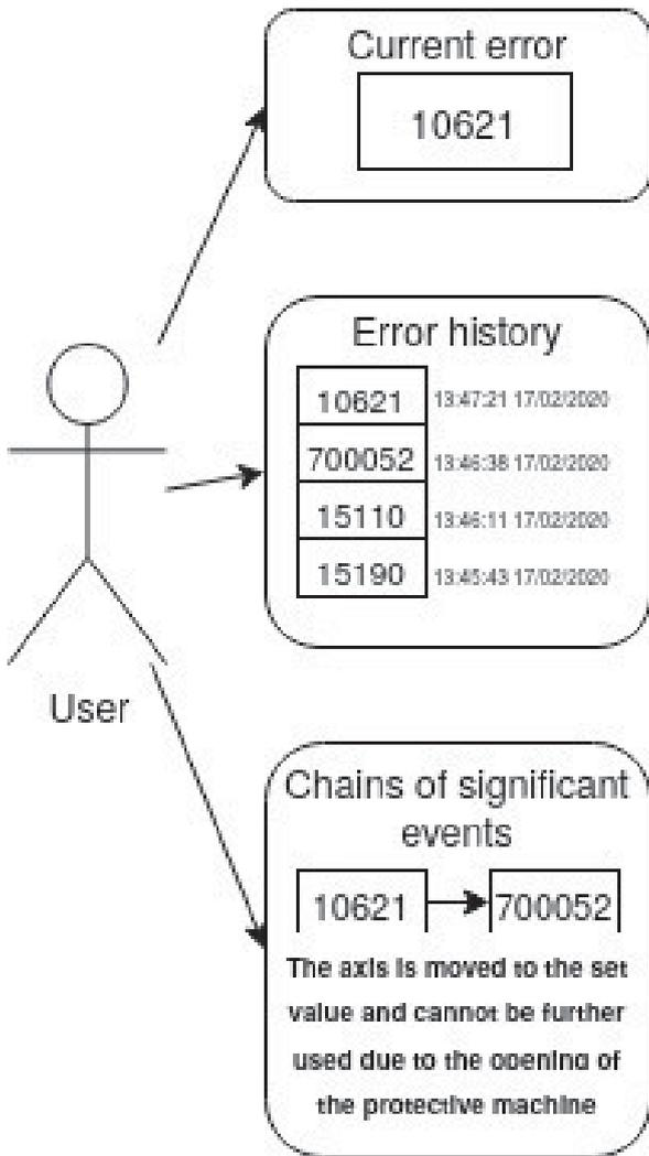
Fig. 2. Options for using the service by the user
