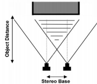
Fig. 2. Schematic representation of a stereophotogrammetric system of two cameras
