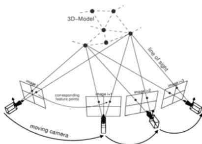
Fig. 1. An example of the Structure from Motion method working for four shots from different positions
