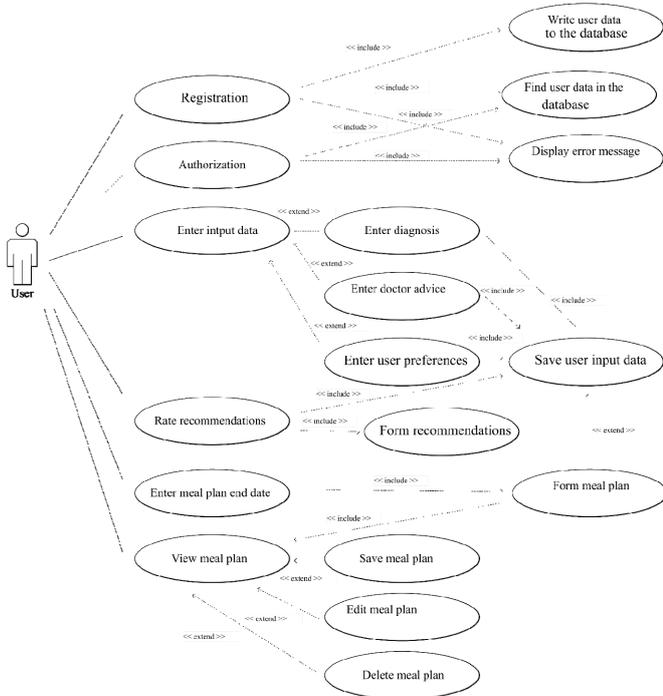
Fig. 8. Generalized use case diagram for the system
