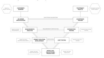
Fig. 2. V-design model of the experimental Smart Factory
