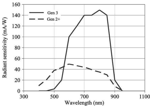
Fig. 2. Color sensitivity of night-vision devices of 2 and 3 generation
