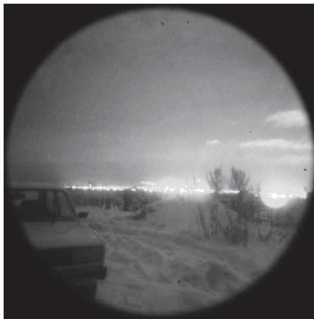
Fig. 1. Example of bloom effect in night vision device. The distance to light sources is about 1.5km
