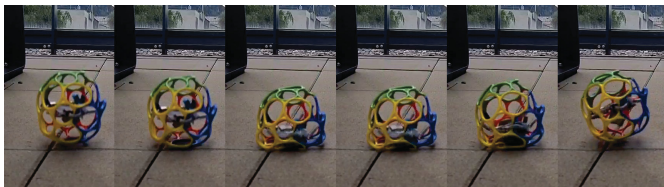
Fig. 9. Deformation of SBS on deployment test from 3m on hard tiled floor — 960 FPS - Frame count of clips 0, 1, 3, 5, 9, 17
