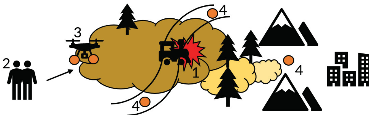
Fig. 1. Overview of the basic concept. 1: location of a train accident with DG forming HG involved, 2: Ground Control for drone operation, 3: UAS detecting boundaries of gas cloud in midair with the sensor; 4: Deployed sensor on strategic locations. Details described in Section III
