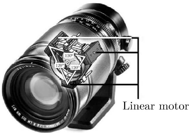
Fig. 2. Shake compensating system (source: https://www.4clik.com )
