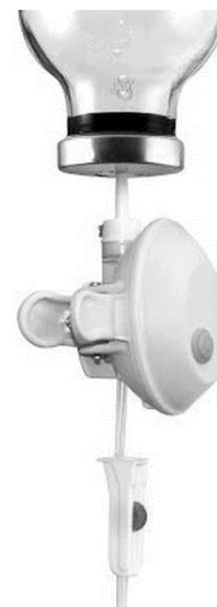
Fig. 7. Autonomous infusion drop counter based on self-mediator software
