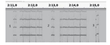
Fig. 3. Clear trace for Alcatel POP3: each time of encryption operation is numbered
