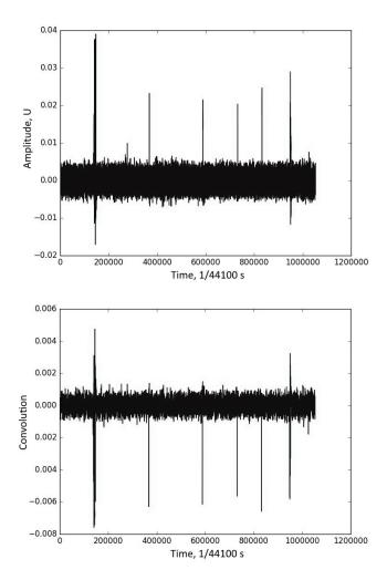
Fig. 7. Signatures detection with the first method
