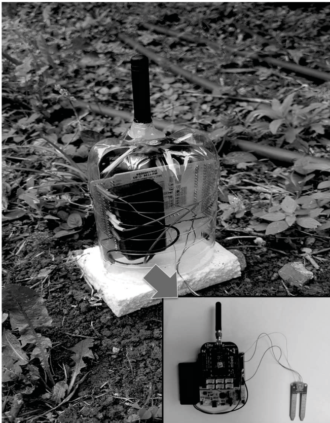
Fig. 4. LoRa device used to measure the soil moisture
