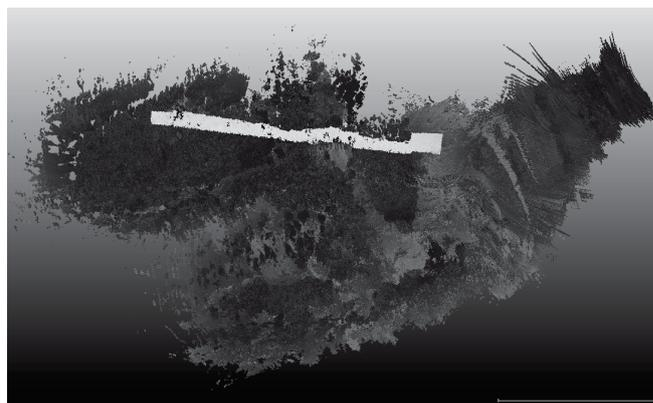
Fig. 13. The region of point cloud (dark points) with the cut (the light line) for exploring the height profile using a zoom
