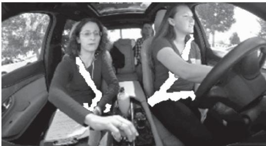
Fig. 2. NADS-Net Output for seat belt segmentation
