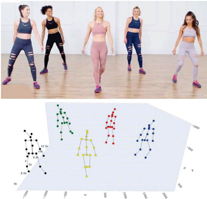
Fig. 6. The result of detecting a three-dimensional skeleton of people in the image
