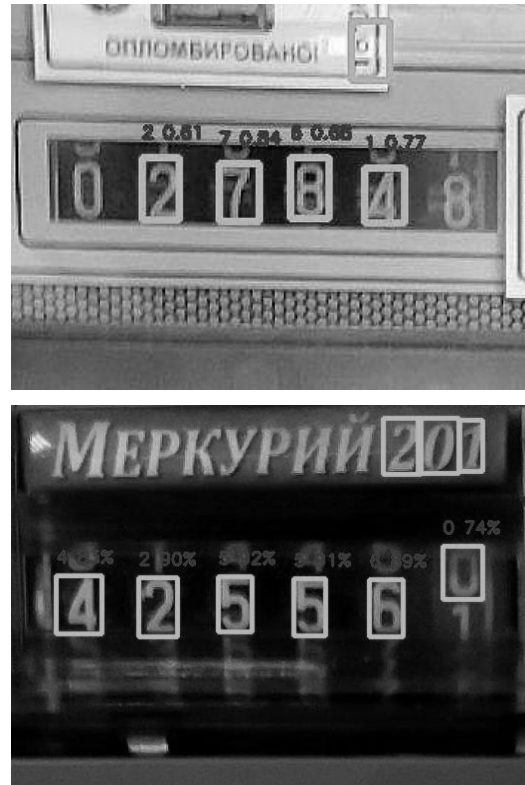
Fig. 5. Examples of real meters reading recognition
