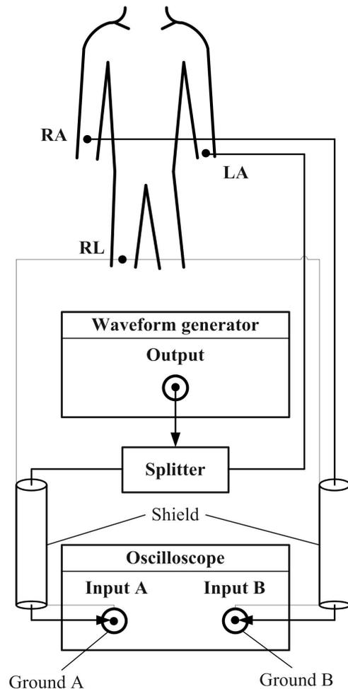
Fig 4. Measurement setup scheme
