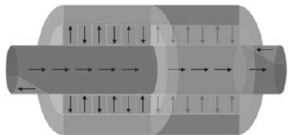
Fig. 3. Domain structure of a magnetic microwire with a dominant central domain (from [24])
