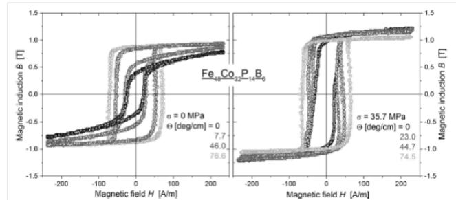
Fig. 2. Dominance of changes of  $M_{rem}$  и  $H_C$  when applying to the Fe<sub>48</sub>Co<sub>32</sub>P<sub>14</sub>B<sub>6</sub> ribbon tension and twisting, respectively [19]
