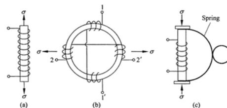
Fig. 1. (a) and (b) are two typical schemes for mounting ribbons as tensile sensors; (c) - design of the compressive force sensor with pre-tensioning spring [6]
