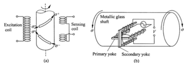
Fig. 5. Designs of the sensors of twisting
