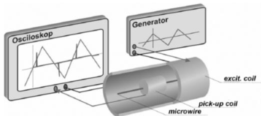
Fig. 4. The scheme for measuring the field of domain switching in a magnetic wire (from [25])
