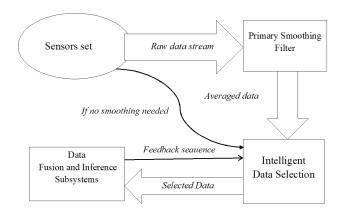
Fig. 1. The sensed data processing
