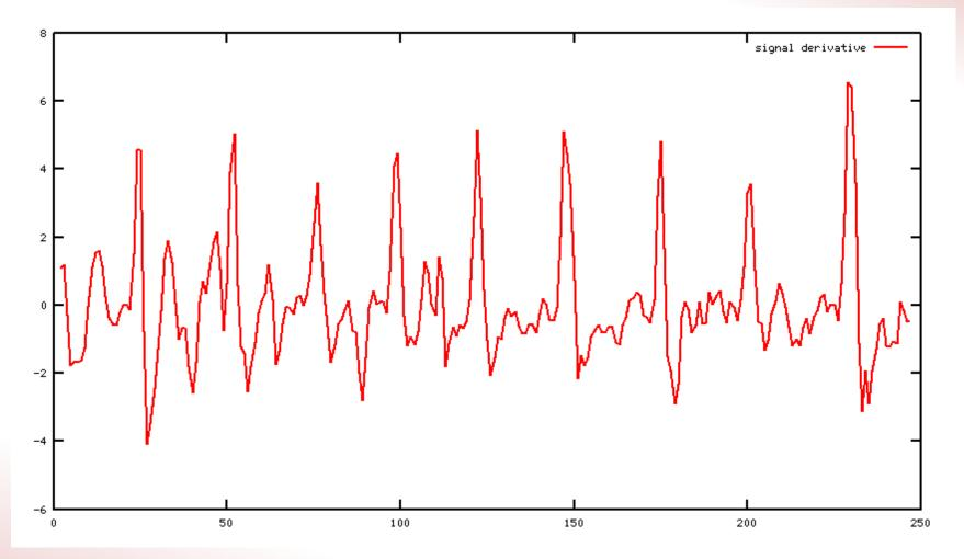
Aligns signal baseline and makes signal's average close to zero
