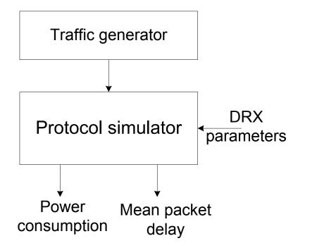
Find parameters corresponding to minimal power consumption under given constraint on delay
