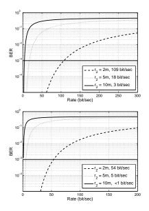
• Uncoded channel throughput (with BER =  $10^{-3}$ ):
